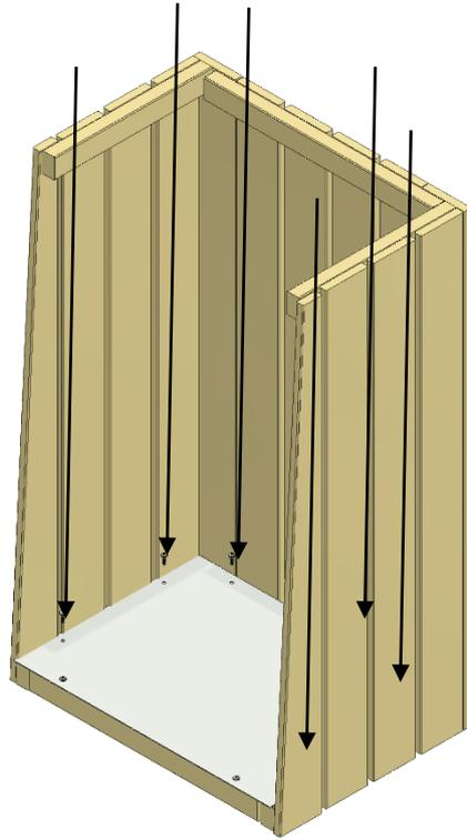
3. Mount the bag lock bracket to the rear panel with screws provided.
