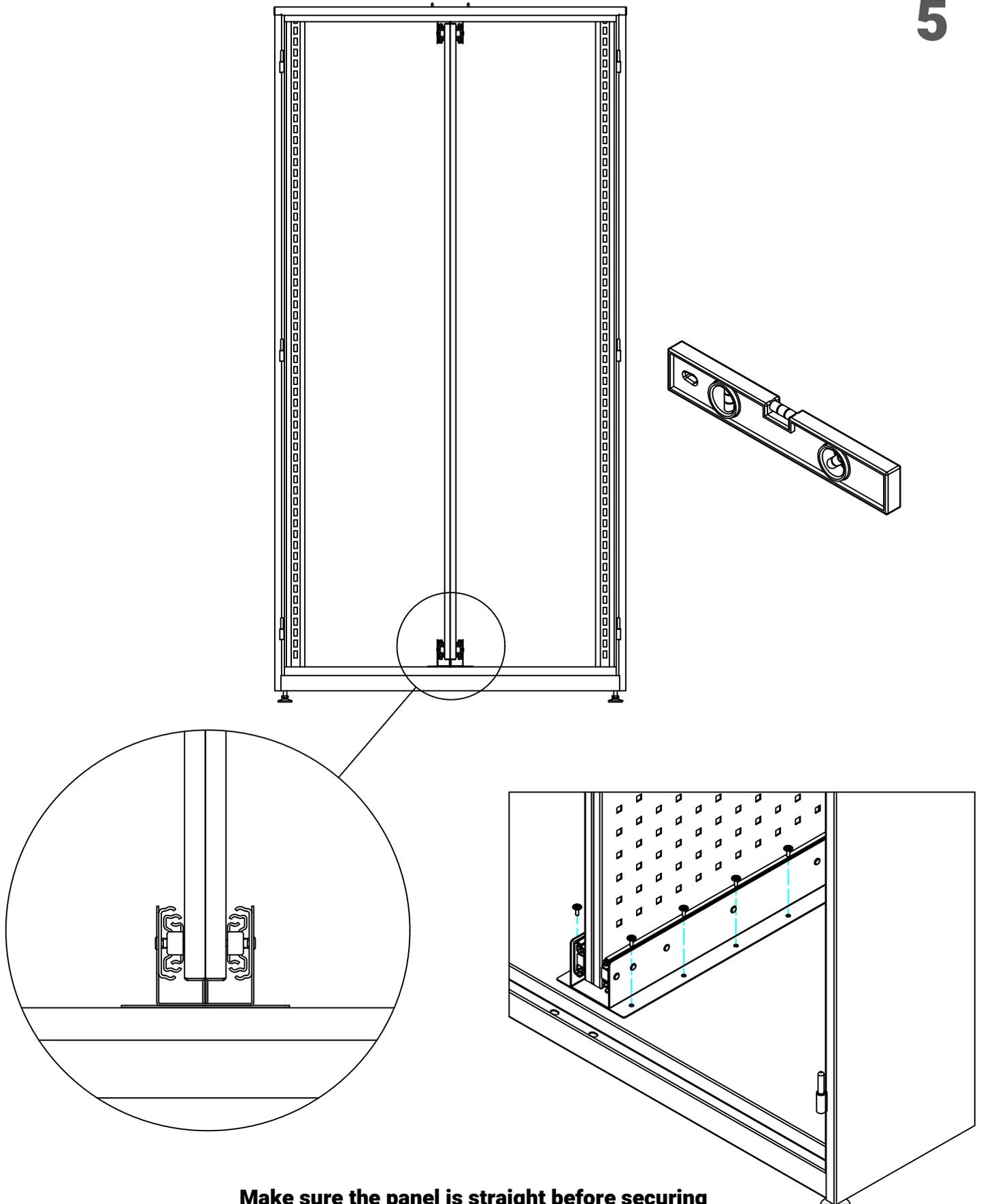
**Make sure the panel is straight before securing the bottom holder with sheet metal screws (10x)**
